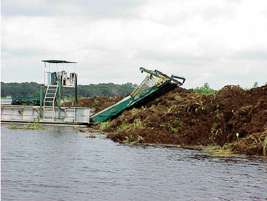
Fig. 10.5 Mechanical removal of floating vegetation in Tsala Apopka Lake, Citrus County, north central Florida ( https://plants.ifas.ufl.edu/manage/why-manage-plants/tussocks-and-floating-islands/ )
