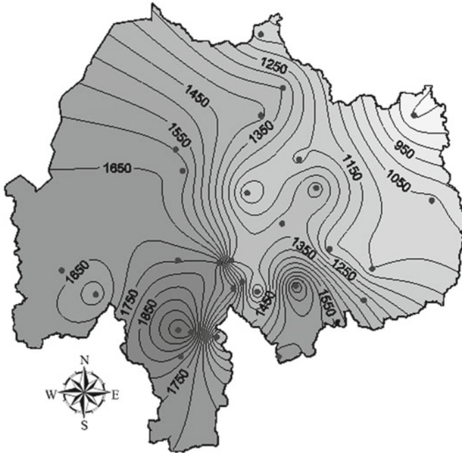
Fig. 4.7 Spatial variation of average annual rainfall on the Blue Nile basin (Abtew et al. 2009b)
