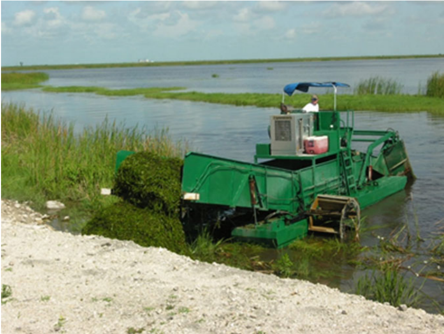
Fig. 10.7 Aquatic vegetation harvester depositing on levee (Photo from South Florid Water Management District)
