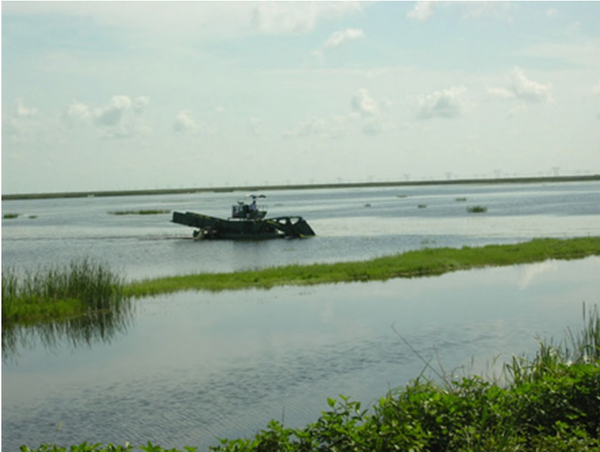
Fig. 10.6 Floating aquatic vegetation harvester (Photo from South Florida Water Management District)
